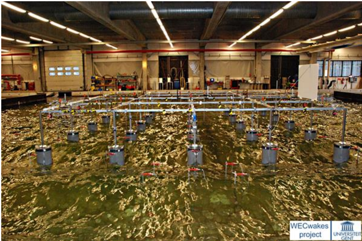
Figure 6: A 5x5 WEC array tested during the WECwakes project (Stratigaki et al., 2014, 2015) at the DHI wave basin within the European Hydralab IV Programme.
